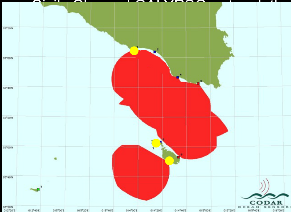
New CALYPSO HFR coverage after installation of 3 additional radars
